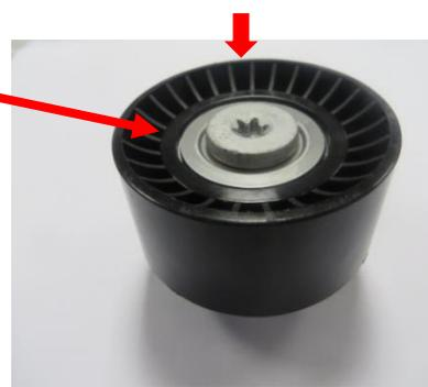
One washer to fit on the bolt head side
