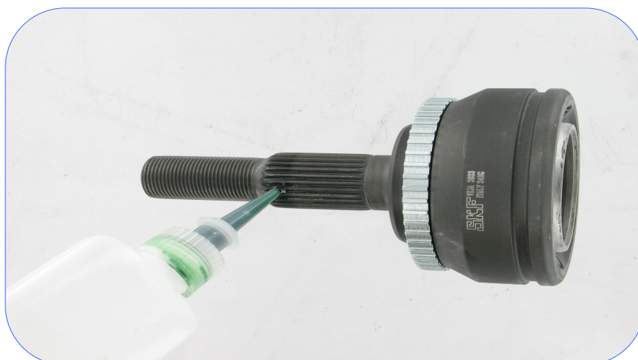
Picture 1: Application of metal glue
