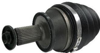
CV-joint / Driveshaft taper with sealing ring
