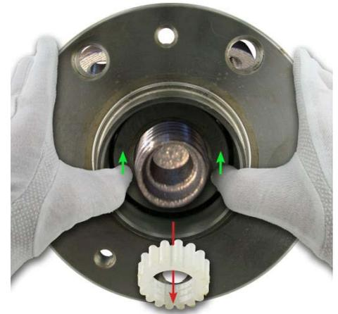
The plastic joining sleeve ring will be automatically pushed out by the axle stub, when mounting the bearing in a correct way, applying the force on the inner ring. Do not push out the plastic sleeve manually before mounting.
