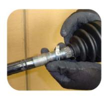
1. Put the short boot clamp on the shaft. Slide the boot onto the shaft.
