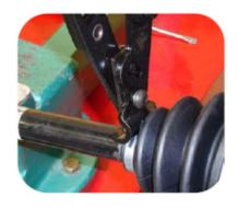
5. Fit the short and long clamps onto the CV-Joint boot and tighten them with a suitable tool.
