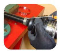
2. Place the driveshaft in a vice (with aluminum or protective jaws). Remove both the inner and the outer clips. Then, cut the boot and remove it.
