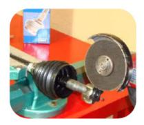
4. Cut the tracks of the inner race, in 2 o 3 positions by using a suitable cutting tool.
