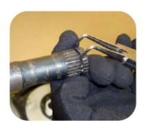
6. Expand and remove the circlip with circlip removal pliers.
