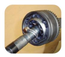
3. Press the new CV-Joint onto the shaft.
