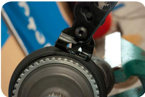
5. Fit the long clamp and tighten it with the same tool.
