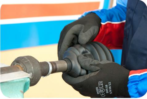
1. Put the short boot clamp on the shaft.
