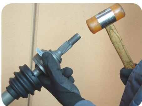
3. Press the new CV-joint onto the shaft.
