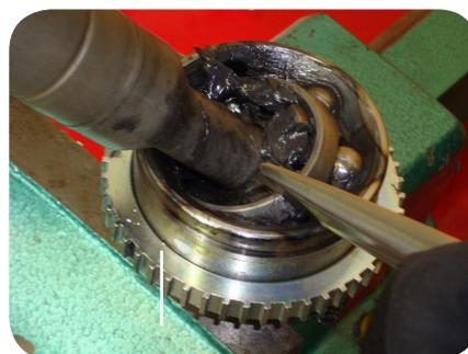
3. Place the CV-joint in the vice. Break the cage in several positions along the edge (close to the balls) using hammer and chisel.
