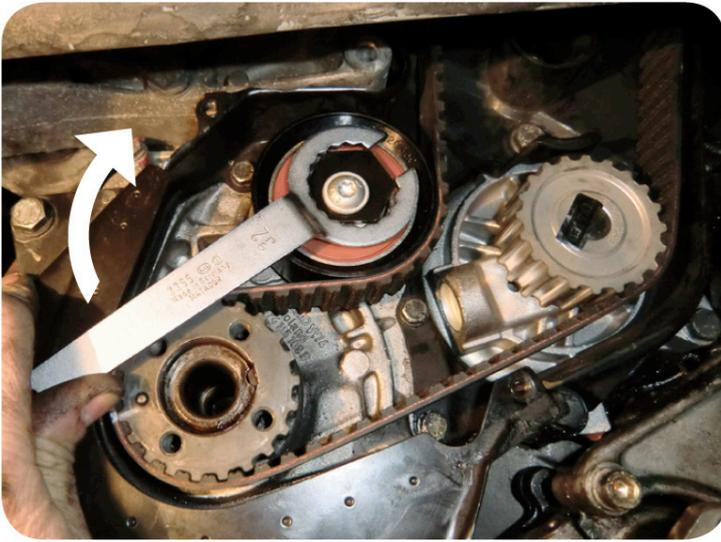
Using the correct tool, rotate the adjuster in a clockwise direction until the pointer is aligned with the center of the backing plate.
