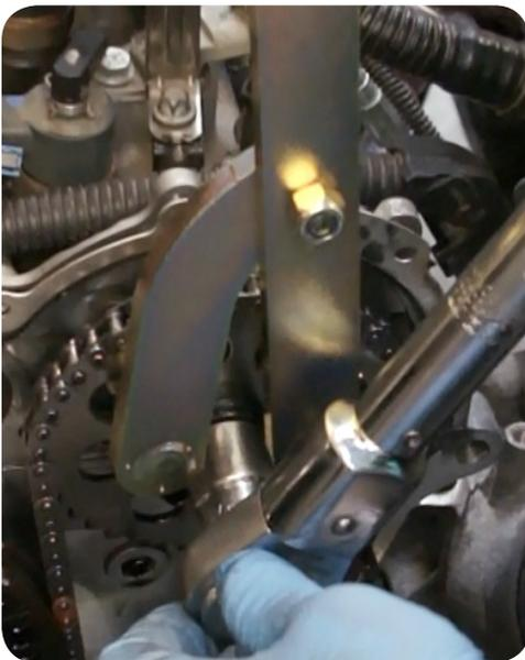
**Attention!** The camshaft sprocket does not have a key slot between camshaft and sprocket. Never use camshaft blocking tool to block the camshaft when removing the camshaft bolt! The high forces could destroy the blocking tool inside the engine and damage the camshaft!
