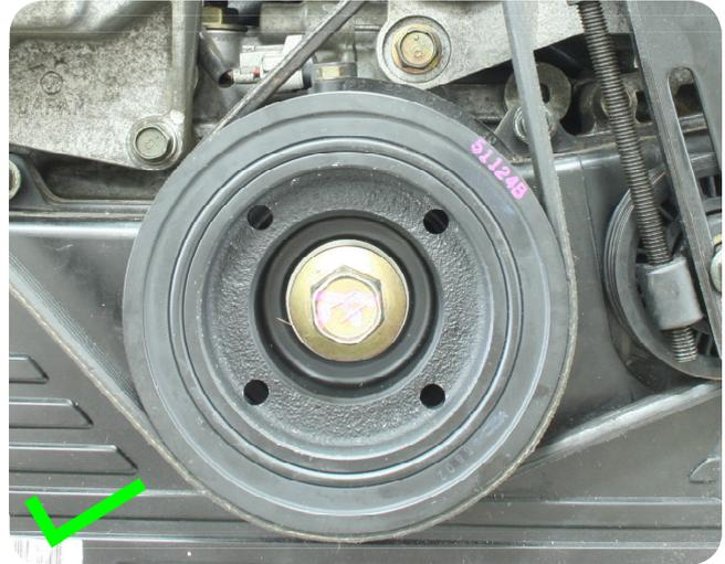
*Aftermarket Power Pulleys vs OE Crankshaft Damper*
