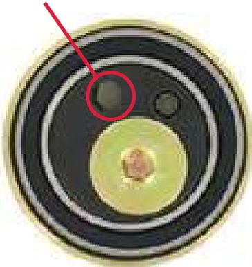
Torque the tensioner fastening bolt to 42 Nm.
