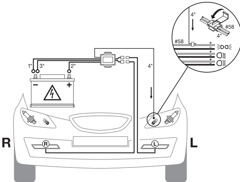
Ⓐ 1 black, 2 red, 3 orange, 4 green. Tip: When you connect the wires, you may connect the orange cable to the battery +, the positive terminal, it can enable the dimming function when switching on position light. This function may only be used in countries where permitted.
