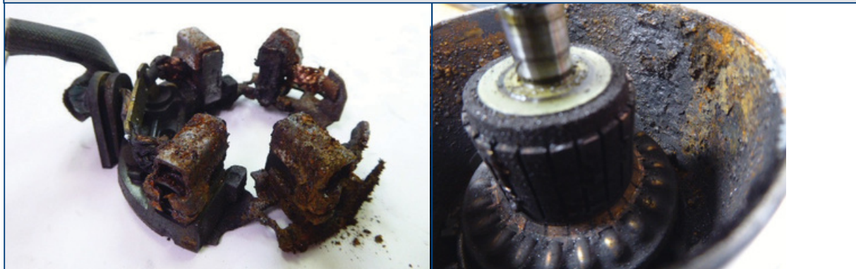
Heavily corroded commutator and armature
