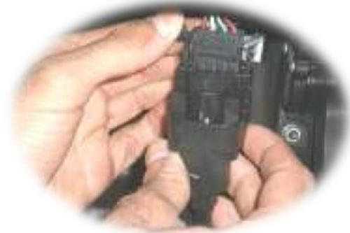
Remove the connector from the brake light switch. To remove the brake light switch, it has to be turned by 45 degrees to the left.
