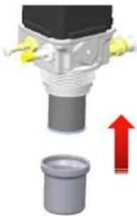
13. The sealing bead of the frost compensation membrane has to be complete, circular and clean in the groove of the pump housing.
