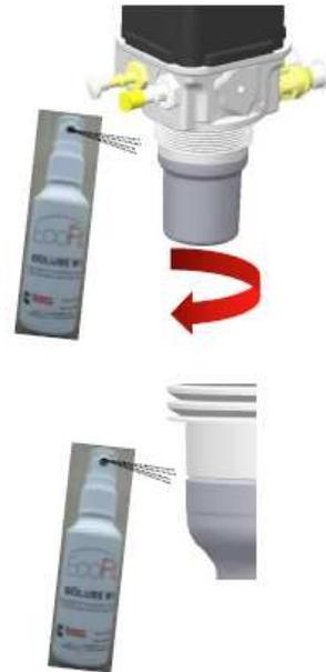
15. The thread on the pump housing needs to be lubricated with Biolube Pump Spray.
