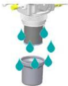
4. Take away the frost compensation membrane off the pump housing.
