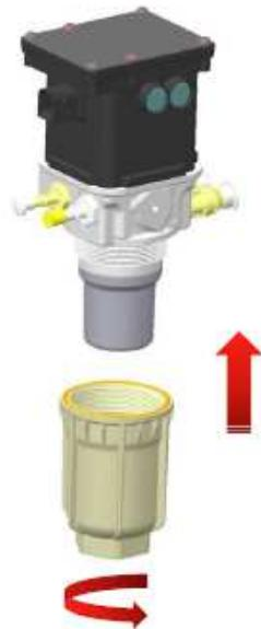
17. Torque the filter housing with torque wrench SW46 to  $80\pm 5\text{Nm}$ .
