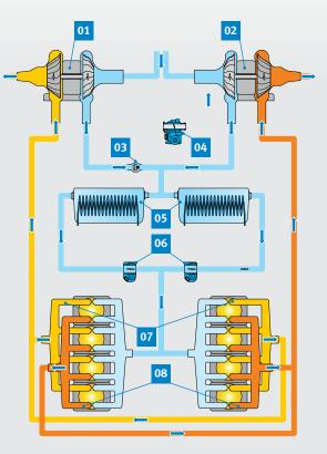
From approx. 2200 rpm, the passive turbocharger (**01**) is activated.
