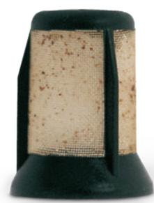
Prefilter of the E3T – blocked by rust
