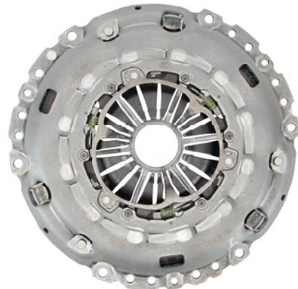
Figure 2: Pressure plate of RepSet 625 3212 09 (for vehicles from model year)
