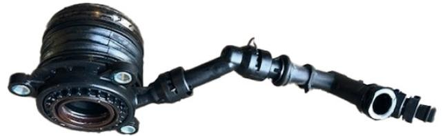
Figure 1: Hydraulic line of the plastic CSC
