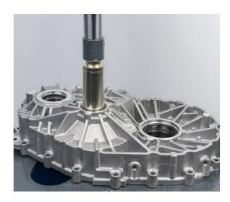
• Press out the drive shaft ball bearing from the gearbox housing
