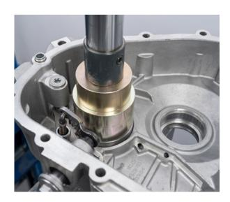
• Press new angular contact ball bearing of the output shaft into the gearbox housing
