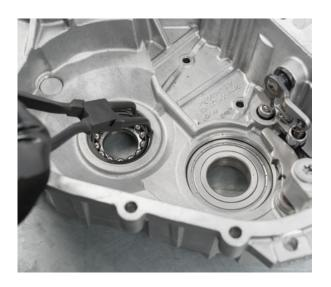
• Press the output shaft angular contact ball bearing out of the gearbox housing
