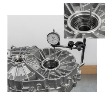
Press the differential gear on the opposite side upward by hand until it stops and read off the measured value
