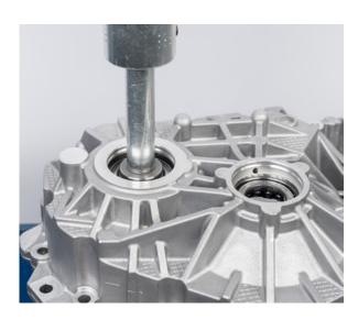
• Remove the retaining circlip for the drive and output shaft bearings
