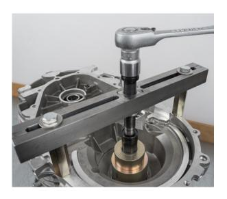
• Press in new shaft oil seal of the differential gear on the motor side
