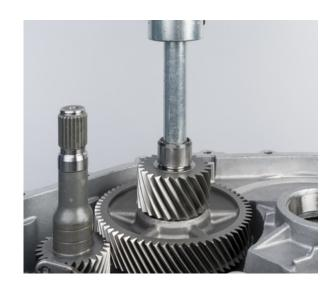
• Insert the differential gear into the motor housing
