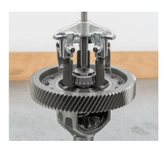
• Press a new tapered roller bearing on the gearbox side of the differential
