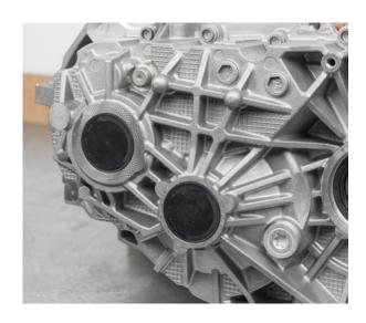
$\bullet$  Install both drive shaft flanges and tighten bolts to 30 Nm
