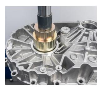
• Press new ball bearing of the drive shaft into the gearbox housing
