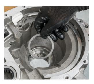
• Press in the new bearing outer race of the differential gear on the motor side
