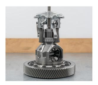
• Remove the tapered roller bearing of the differential gear on the gearbox side
