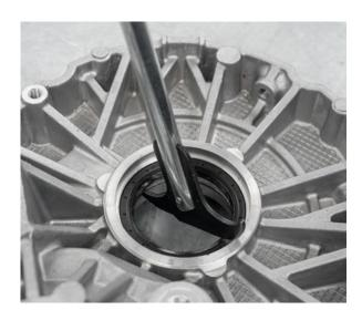
• Remove the bearing outer race from the gearbox side using a suitable internal extractor
