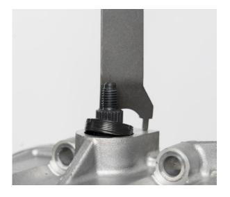
• Mount new oil seal with suitable sleeve to previous installation depth
