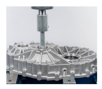
• Press out the drive shaft from gearbox housing
