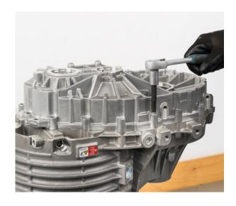
• Lift gear housing evenly upwards
