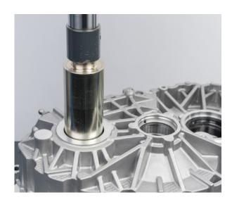
• Remove the drive flange oil seal from the gearbox side
