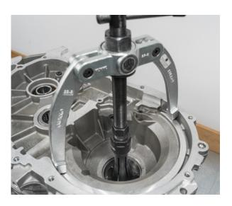
Press in new motor-side bearing outer race of the differential gear <u>without</u> the adjusting shim
