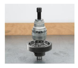
• Remove the motor-side bearing inner ring on the output shaft as described in the next step
