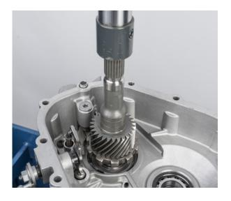
Press the drive shaft into the gearbox housing
