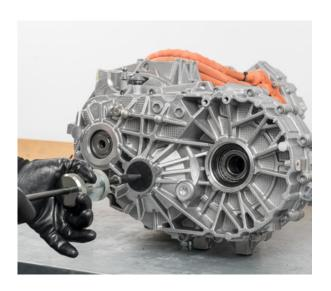
• Remove the retaining circlip for the drive shaft
