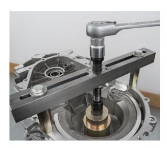
• Remove the tapered roller bearing of the differential gear on the motor side
