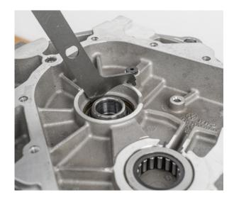
• Press in new shaft oil seal for the rotor shaft to previous installation depth
