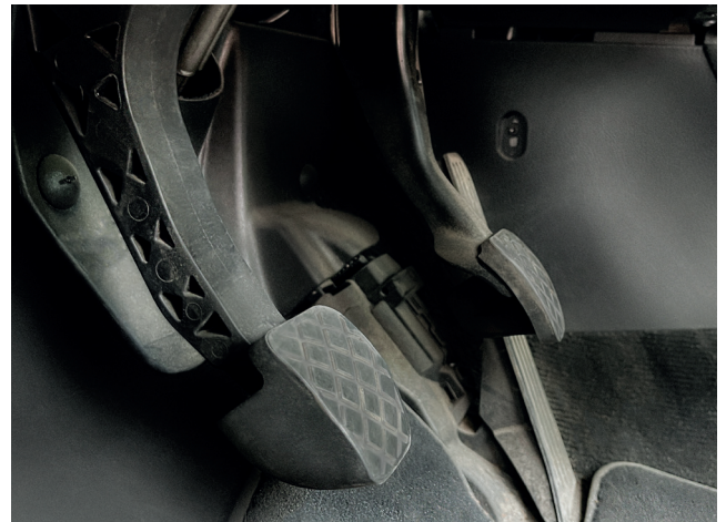
Image 1: The clutch pedal hanging up in the middle of its travel
