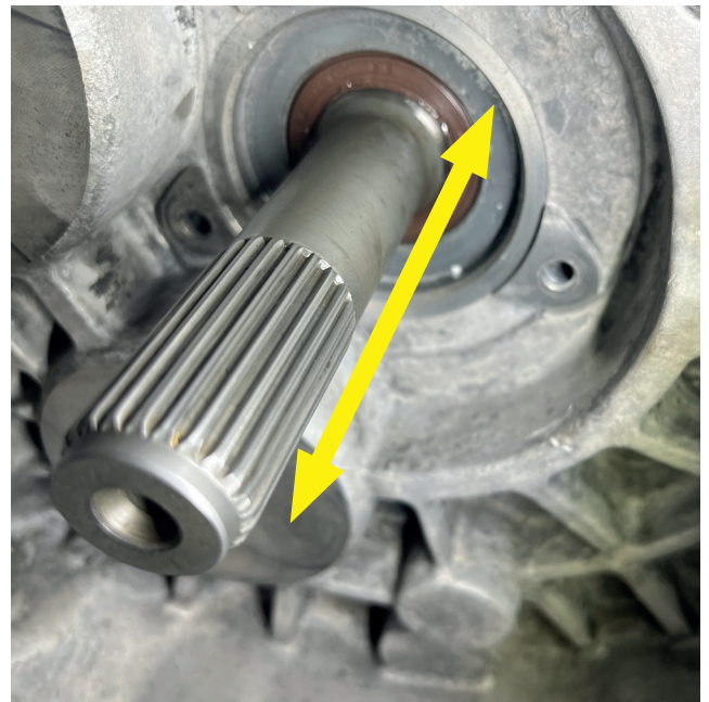
Image 2: Axial clearance of the gearbox input shaft
