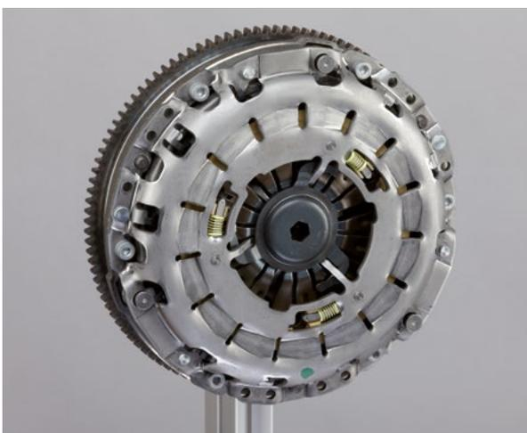
Clutch pressure plates on some BMW models are equipped with a locking device which makes the use of a conventional centring pin impossible. This is why a special pin design or centring sleeve is required.
