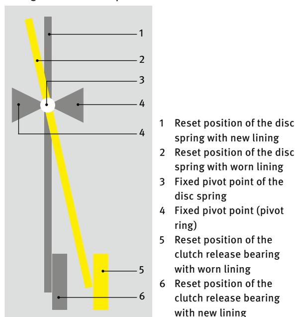
These challenges were reason enough to turn to a new type of solution. The foundations were set for the development of the self-adjusting clutch.
