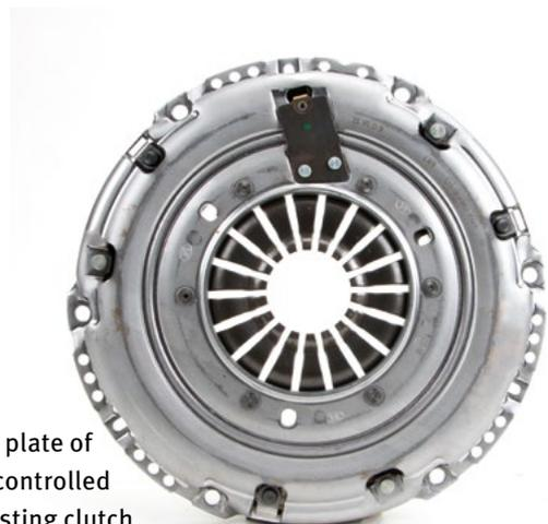
Pressure plate of a travel-controlled self-adjusting clutch
