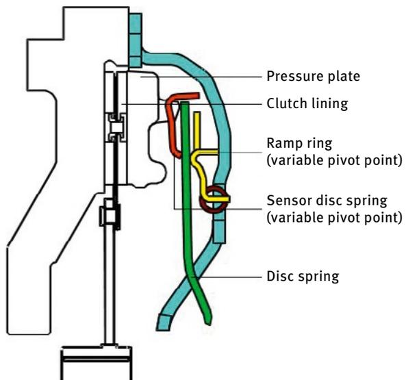
The travel-controlled self-adjusting clutch uses changes in the pressure plate travel to adjust the pivot points of the disc spring if wear has occurred. Force and travel-controlled pressure plates are used by reputable vehicle manufacturers. This brochure describes the structure and function of both self-adjusting clutch systems.
