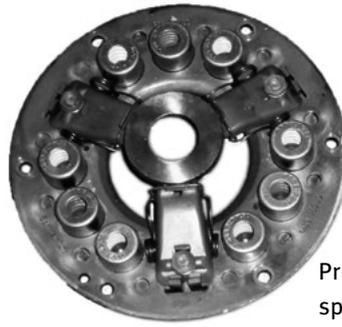
Pressure plate of a coil spring clutch
