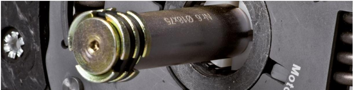
Correct assembly of the centring pin is dependent on the inner diameter of the pilot bearing or crankshaft bore, and on the distance between the pilot bearing or crankshaft bore and the clutch disc's hub profile.
