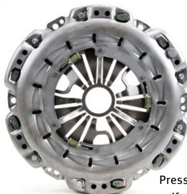
Pressure plate of a self-adjusting clutch
