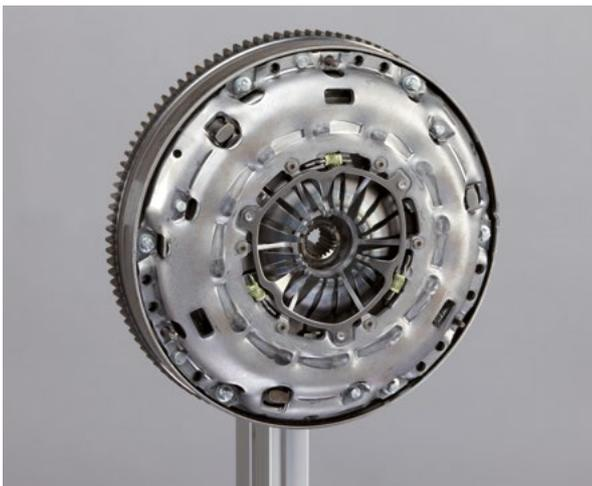
If a certain repair procedure requires the SAC to be disassembled and then re-installed, it is essential to use a special tool as this is the only means to ensure full operational reliability of the part after re-installation.
