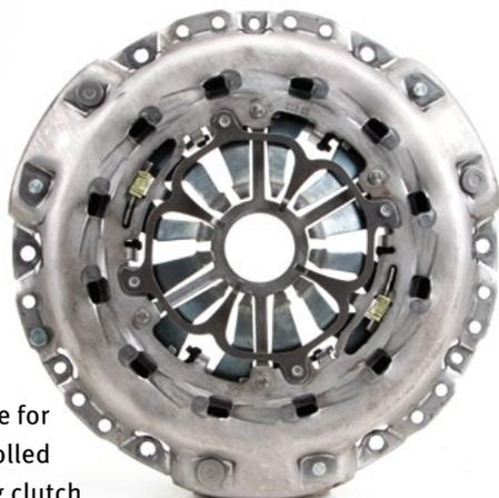
Pressure plate for a force-controlled self-adjusting clutch
