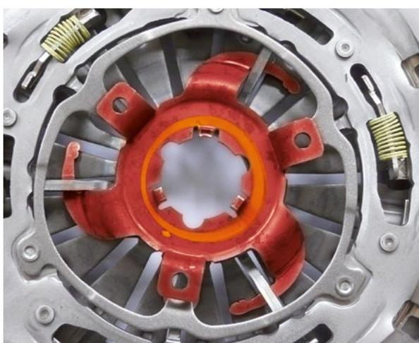
Clutch pressure plates for these models can be equipped with a locking device. The clutch disc is centred by means of the universal centring pin.
