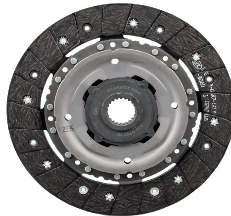
Fig. 2: Clutch disc with hub damper (diameter 228mm or 240mm)
