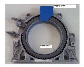
The crankcase is sealed on the flywheel side by sealing flange with PTFE sealing ring and sender wheel
