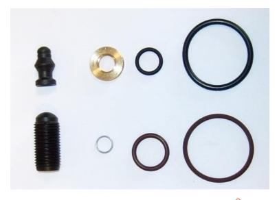
Always replace the adjusting screw as well when exchanging the ball pin. The Elring seal kit, injection nozzle 900.650 contains both components for this purpose. In addition to resulting in far greater wear, the use of an old and worn adjusting screw together with a new ball pin vastly increases the risk of ball pin fracture. Please avoid fitting an old adjusting screw in combination with a new ball pin.
