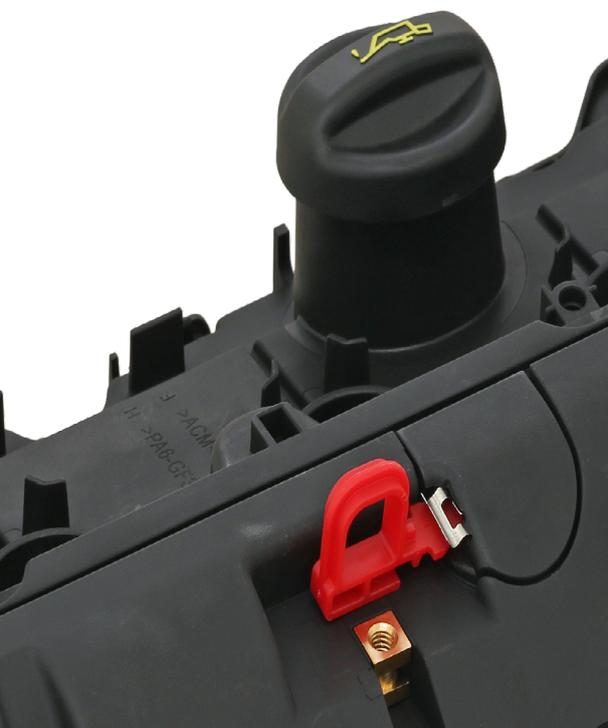
The maintenance tool is used to unlock the cover of the crankcase ventilation unit (control valve) and is only needed in the event of repairs, e.g. to remove contaminants.
