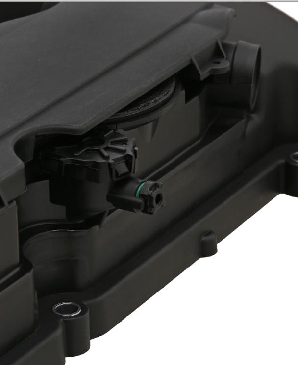
In the case of vehicle models that have been specially manufactured for the Korean or American market, the open valve plug has to be mounted instead of the red sealing plug. Can be seen in the image on the left.
