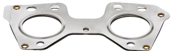
Firstly, a three-layer metallic layer sealing system with patented half bead using Metaloseal™ L from ElringKlinger as the initial material. This is backed up by a molybdenum disulfide / graphite based sliding lacquer on the side facing towards the exhaust manifold. Finally, a high temperature resistant resin binder is added and is primarily intended to reduce frictional wear.
