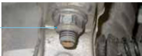
**!** To protect the thread, leave the nut a few turns on the pin.
