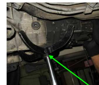
Use the appropriate device to assembly and disassembly the gearbox. The operator never must support the weight of gearbox.
