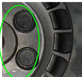
Multiple holes washer assembled detail
