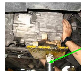
Use the appropriate device to assembly and disassembly the gearbox
