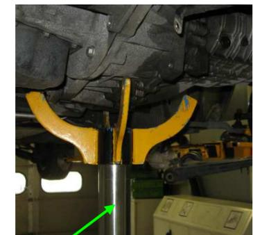
Use the appropriate device to assembly and disassembly the gearbox. The operator never must support the weight of gearbox.
