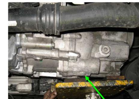
Use the appropriate device to assembly and disassembly the gearbox. The operator never must support the weight of gearbox.
