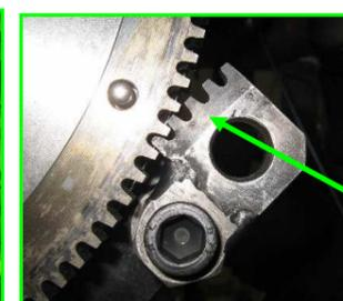
Use a device to block the flywheel during tightening operations
