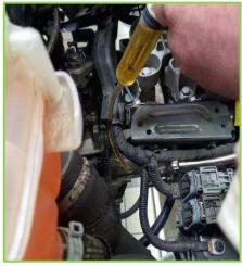
**STEP 7 - Bleeding procedure**Inject brake fluid via CSC purge valve until to see rise of the brake fluid in the reservoir.
