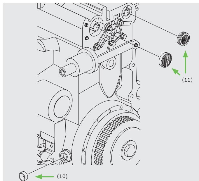
At some vehicle models, the camshaft pulleys will have to be loosened when installing the new timing-belt kit.
