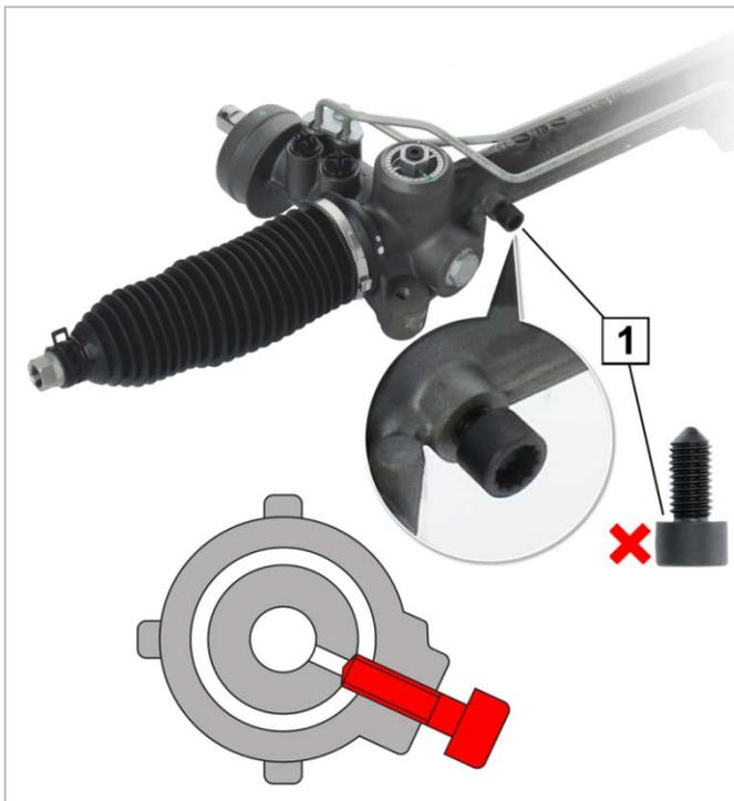
Fig. 3: Screw for steering center alignment
