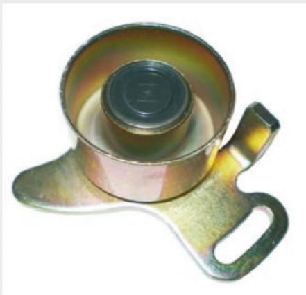
**Novi zatezni valjak s pločom**
