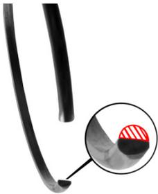
Fig. 3: Worn retaining ring.
