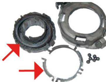
Fig. 4: Mechanical damage and overheating on the releaser
