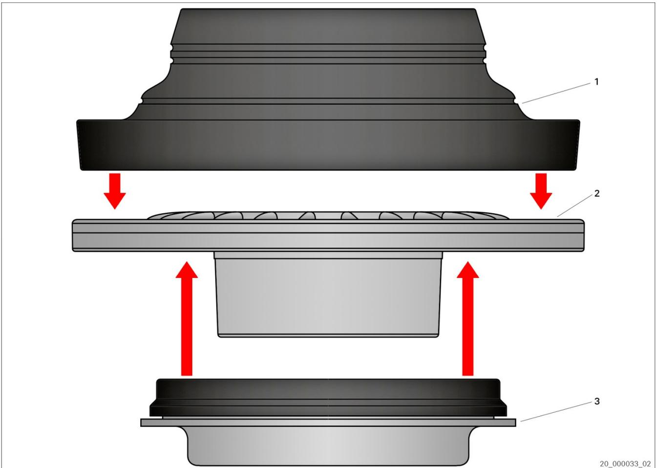
Fig. 1: Assembly of the suspension-strut mount (example)
