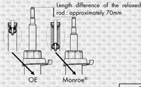
In order to ensures a better quality and better longevity, Monroe® brings improvements in the manufacturing process of these shock absorbers : inner buffer is substituted by a rebound spring.
