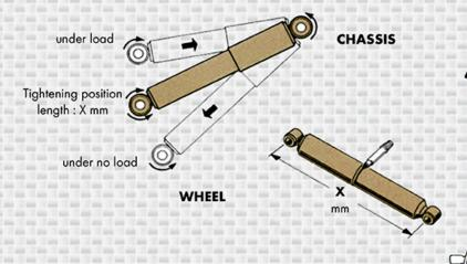
To facilitate installation, refer to chart bellow, mark a reference guide when the correct length (X) is achieved on the new shock absorber. The reference line should be used as a guide during the installation process. Ensure the reference line lines up whith the dust shield before tightening the mounting bolts
