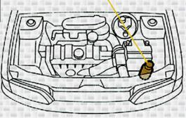
Identification of a vehicle with power assisted steering
