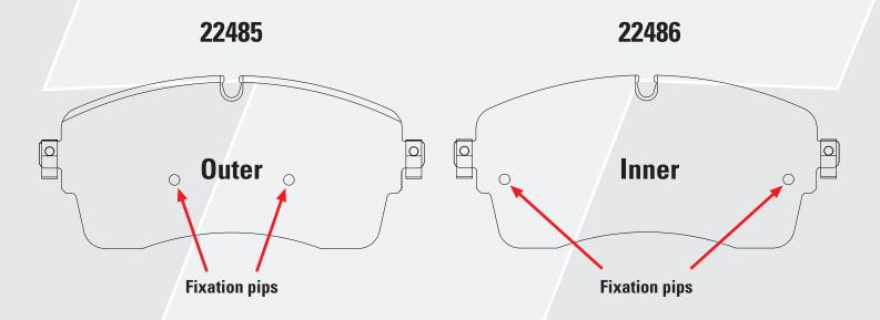
Due to these different locations of the pips, the parts are not interchangeable in the caliper. WVA 22485 is for the outer side, 22486 is for the inner side. Swapping the sides of these parts would cause the piston or respectively the fingers of the caliper to push against the pips. This could result in noise issues or an uneven wear of the friction material. Therefore, please look at the brake pads carefully to ensure that they are not mixed up prior to assembly.
