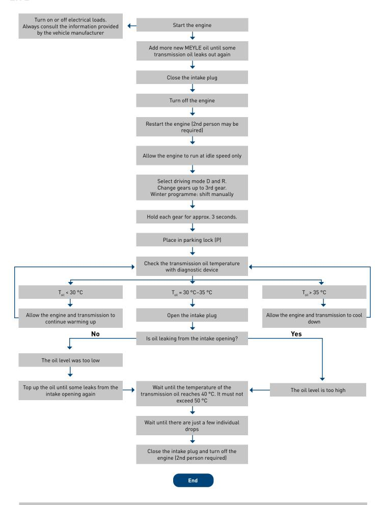
NB: Depending on the type of transmission, it may have a bypass valve which opens or closes the oil circuit to the oil cooler, which is why the drive should be sufficient to ensure the transmission oil temperature reaches at least 75 °C.
