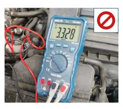
If you measure a voltage of approximately 3.3 V, the glow plug is not compatible with this vehicle.
