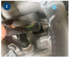
You can identify the pressure sensor glow plug by the fact that a 4-pin connector is attached to it.
