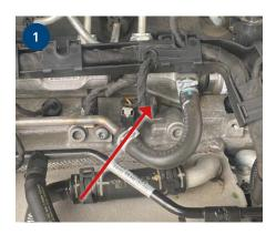
When it comes to 4-cylinder VAG engines, the pressure sensor glow plug is installed at the third cylinder.
