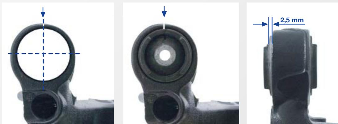
The slot in the new rubber mount must be aligned with the marking on the trailing arm, then installed with a suitable special tool until the mounting is pressed in, up to the dimension of 2.5 mm.
