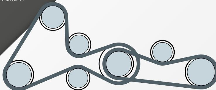
Fig 1 - Auxiliary drive diagram (up to and including engine No. 0113089), fitted with tensioner pulley 37 93 0167 and multi V-ribbed belt 37 92 8798.
