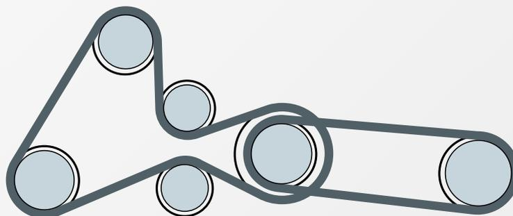
Fig 2 - Auxiliary drive diagram (from engine No. 0113090), fitted with the elastic multi V-ribbed belt 70 94 0717.
