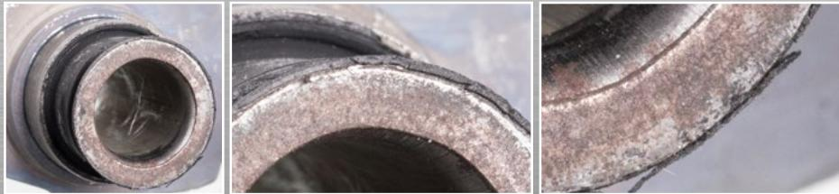
EN Mechanical manipulation of the bearing surfaces removes the corrosion protection. This treatment is carried out in order to enlarge the contact surface of the screw. The presence of rust depends on the period of storage / atmospheric humidity and does not have an adverse impact on the working of the products. Subsequent application of protection to the surfaces can result in impairment of the function.
